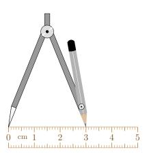
3. Place the needle of your compass on point O. Hold the compass steady and rotate the pencil around O to draw the full circle with a radius of 3 cm.
