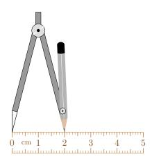
3. Place the needle of your compass on point O. Hold the compass steady and carefully rotate the pencil around O to draw the full circle with a radius of 2 cm.
