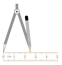
3. Place the needle of your compass on point O. Hold the compass steady and carefully rotate the pencil around O to draw the full circle with a radius of 2.5 cm.
